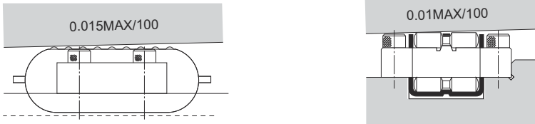
(a) Parallelism between the LM Roller and the raceway (b) Allowable tilt of the roller in the longitudinal direction
