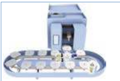
Machine tool Automatic pallet pool drive
