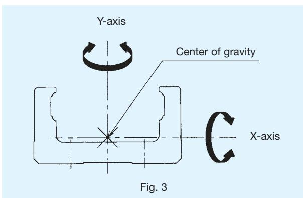
The U-shaped cross section of the rail contributes to weight reduction and minimises deflection. Thus, the LM Guide Actuator can support a load on one side as well as on both.
