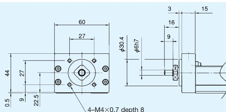
Fig. 14 KR33 Housing A without motor flange (Specification □ 40)
