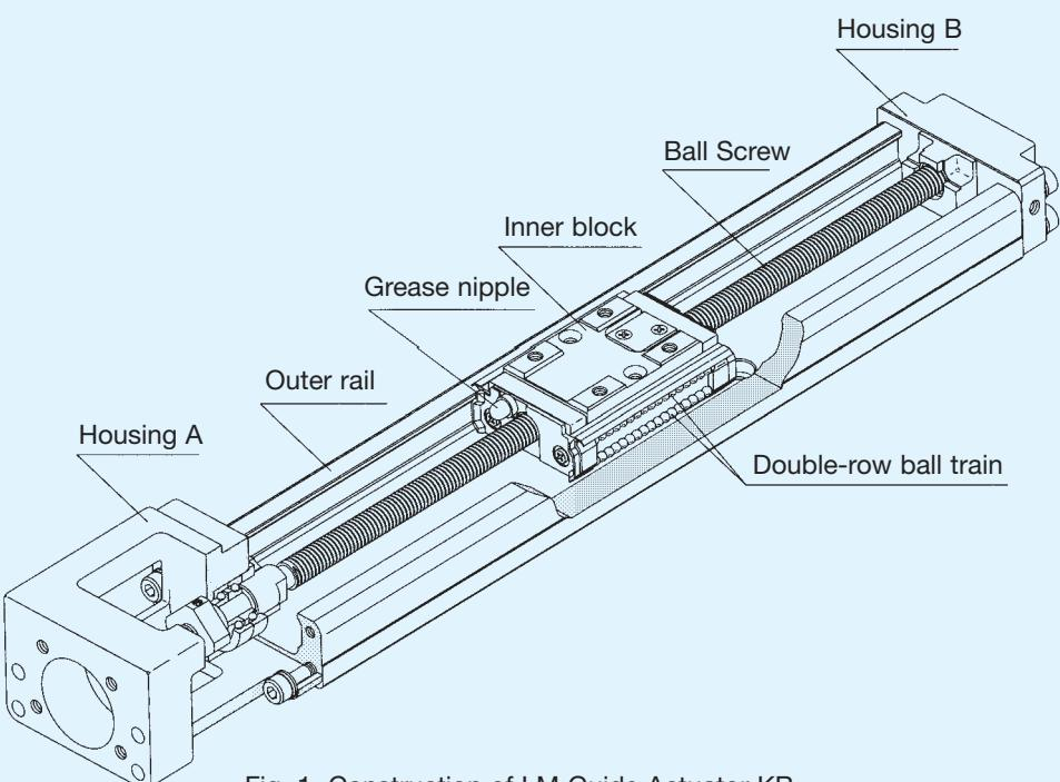
Fig. 1 Construction of LM Guide Actuator KR
