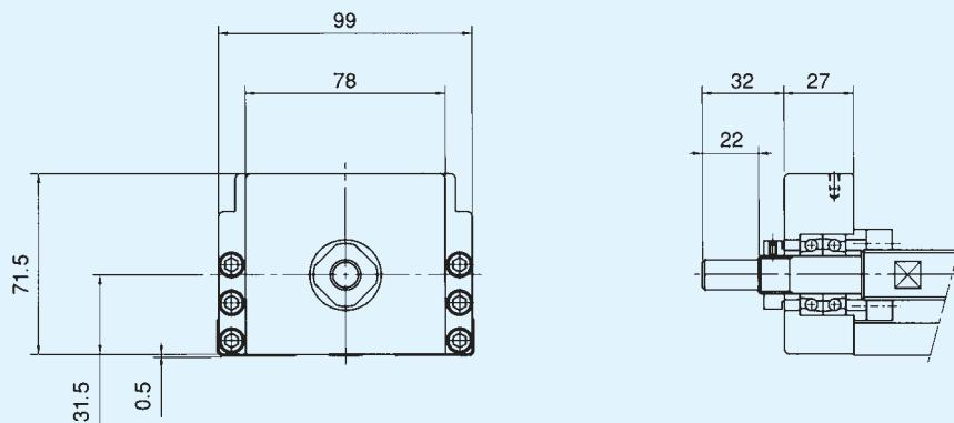
Fig. 17 KR55 Housing A without motor flange (Specification □□10)
