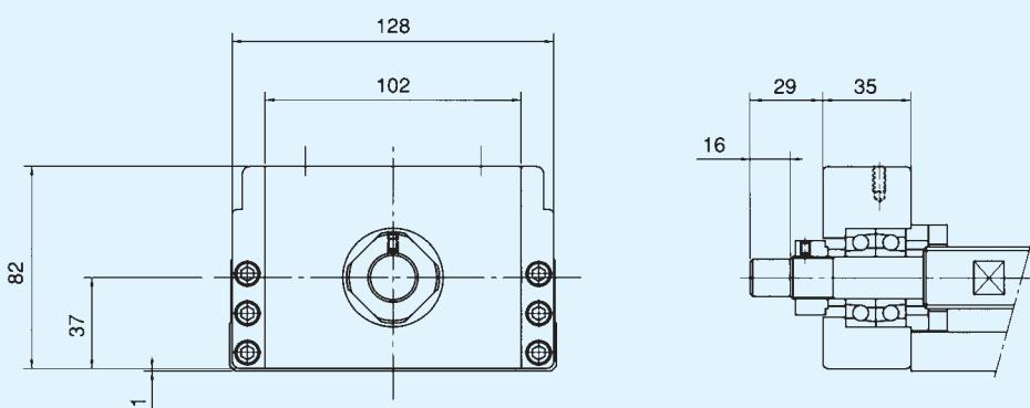
Fig. 18 KR65 Housing A without motor flange (Specification □□10)
