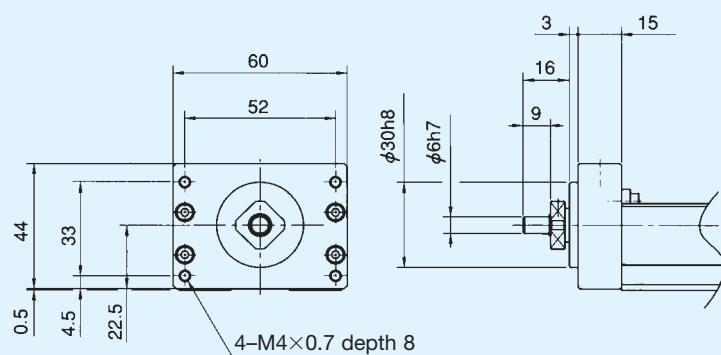
Fig. 13 KR33 Housing A without motor flange (Specification □ 30)
