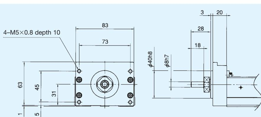
Fig. 15 KR46 Housing A without motor flange (Specification □ 50)
