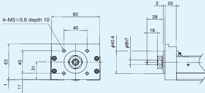
Fig. 16 KR46 Housing A without motor flange (Specification □□ 60)
