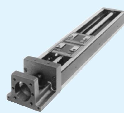
Built by adding another inner block to type KR-C. Permits a span best suited for the host system, thereby enabling higher rigidity to be obtained.
