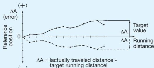
Fig. 11 Positioning Accuracy
